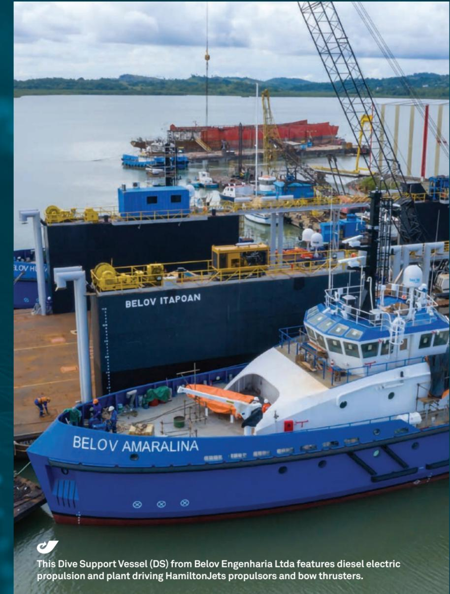
This Dive Support Vessel (DS) from Belov Engenharia Ltda features diesel electric propulsion and plant driving HamiltonJets propulsors and bow thrusters.
