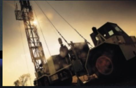
This 115-ton (gvw) Liebherr MPC (Multi-Purpose Carrier) 12x12 is equipped with an MTU 905-horsepower engine and a Twin Disc TD101-3600 10 Speed Automatic Transmission with FLW-1854-1 Torque Converter and an ETA28N Electronic Control.
