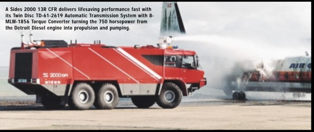
A Sides 2000 13R CFR delivers lifesaving performance fast with its Twin Disc TD-61-2619 Automatic Transmission System with 8-MLW-1856 Torque Converter turning the 750 horsepower from the Detroit Diesel engine into propulsion and pumping.
