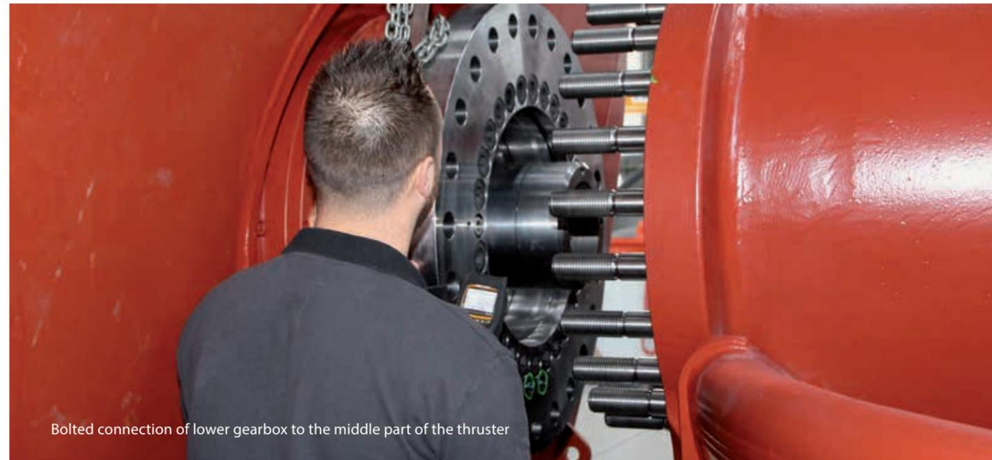
Bolted connection of lower gearbox to the middle part of the thruster
