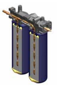
The flow is split between the two filters shown. Half of the flow travels through the first filter and the remaining flow travels through the second filter. Flow does not travel through both filters in sequence.
