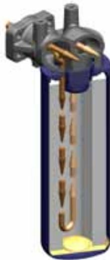
Clean fluid is pushed out of the filter, through the head and out into storage or for use.
