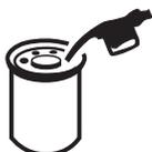
When filling a filter with liquids remember to add the oil, fuel or coolant to the "dirty side" of the filter. Don't make the mistake of pouring unfiltered liquid down the filter center tube.
