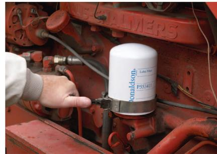
To avoid cross-threading DO NOT OVER TIGHTEN OR RETIGHTEN a filter.
