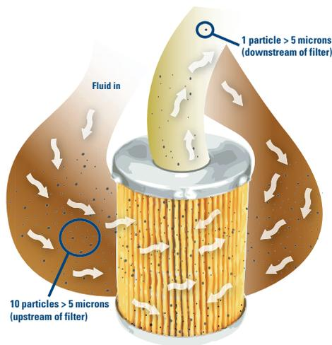
The formula used to calculate the beta ratio is:
