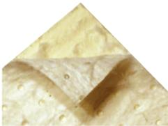
This multiple-layered media technology is designed specifically to remove contaminant AND water from the fuel stream.
