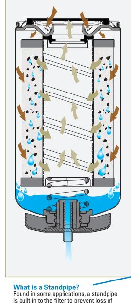
system prime to reduce or eliminate air from reaching the fuel injection system. Clean fuel enters the filter through holes in the baffle/thread plate.
