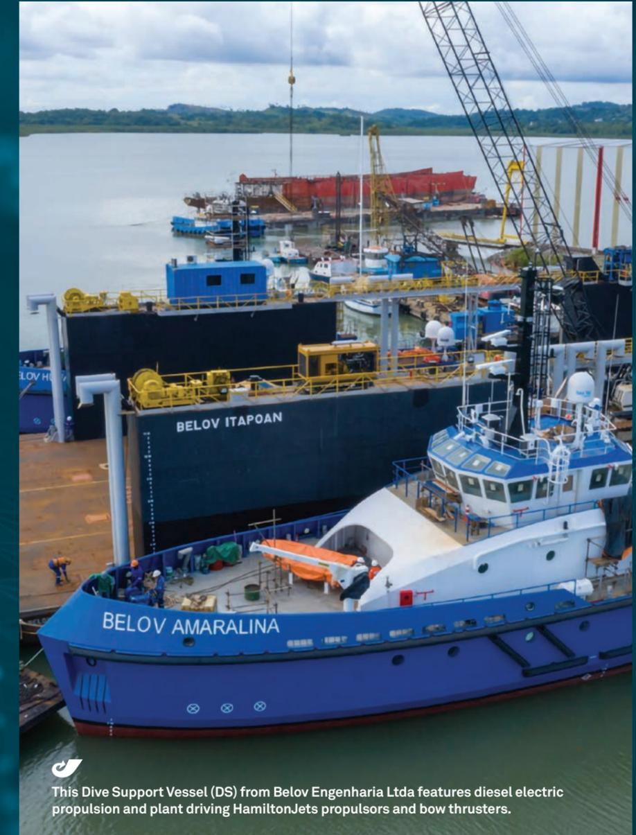
This Dive Support Vessel (DS) from Belov Engenharia Ltda features diesel electric propulsion and plant driving HamiltonJets propulsors and bow thrusters.
