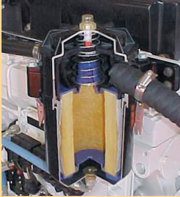
Cummins QSM11 marine engine with CCV cutaway
