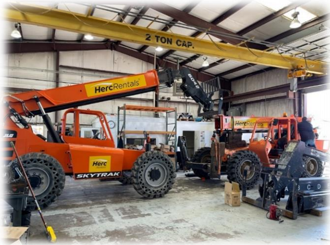
Removing the twisted Boom Sections for repair.
