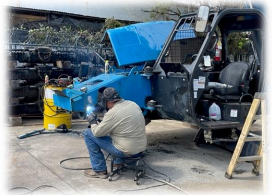
Welder installing new plates on this Genie.
