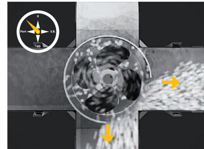
For our 2-channel version we have developed a system in which the steering angle of the drum and the speed of the diesel engine is continuously variable in a setup using one infinitely adjustable handle (which moves from side to side, like a tunnel). The operation is thus highly effective and very responsive!
