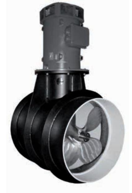
On our tunnel thrusters, we use a standard stainless steel pipe band in the tunnel at the height of the propeller. This makes our tunnel thrusters robust, durable and safe.
