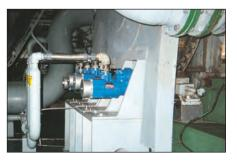
A multiple-starter application on a Clark TCV-12 lowered air consumption by 40% over competitive turbine starters originally applied.
