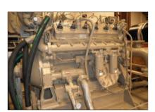
T106-F installed on Caterpillar 3412 engine.
