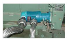
T50-P installed on Caterpillar 3516 engine.
