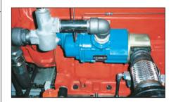
Pressure check ports on both starter inlet and exhaust allow easy troubleshooting of compressed starting air/gas supply valves, filters, piping, and regulators. (Shown here TurboTwin Model T100-V and TurboValve.)
