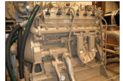
T106-F installed on Caterpillar 3412 engine.
