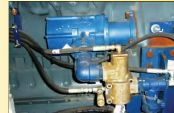
T100-F installed on Detroit Diesel 16V2000 engine.
