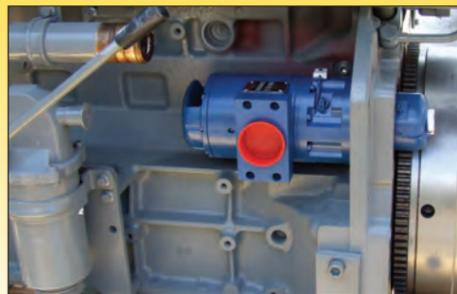
T20 installed on Deutz 1013 engine.
