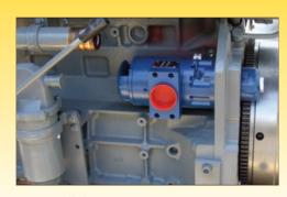
T20 installed on Deutz 1013 engine.
