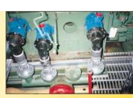
A trio of T100-Ds on a Clark gas engine provide the reliability to handle the higher cranking speeds.
