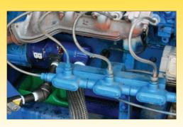
T20 installed on 5.9 Cummins engine.
