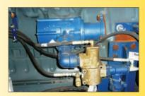
T100-F installed on Detroit Diesel 16V2000 engine.
