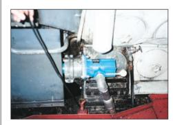
Two views of a T100-D on an EMD 16-567 diesel engine
