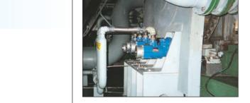
A multiple-starter application on a Clark *TCV-12 lowered air consumption by 40%* over competitive turbine starters originally applied.
