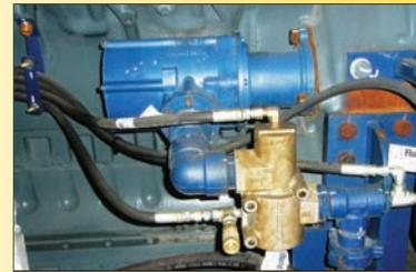
*T100-F installed on Detroit Diesel 16V2000 engine.*
