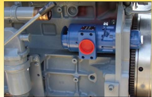
T20 installed on Deutz 1013 engine.
