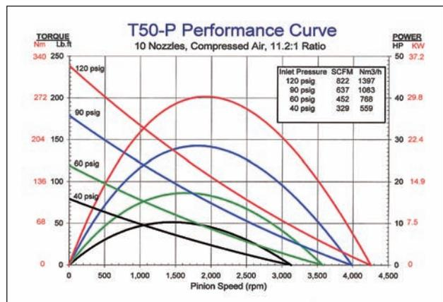
At 34 lbs. and 6" in diameter, the compact T50 delivers 40 hp of cranking power.
