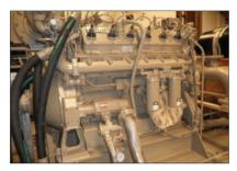
T106-F installed on Caterpillar 3412 engine.
