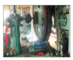
Model T100-B outboard-mounted starter on a slow-speed spark-ignited engine.
