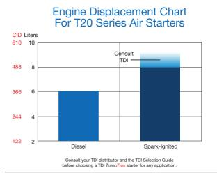
This selection chart shows basic starter capability by engine size. Note the chart shows four-stroke diesel engine size on the left and fourstroke, spark-ignited engine sizes on the right. Always consult TDI for applicationspecific capability.
