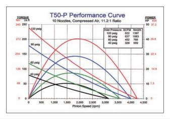
At 34 lbs. and 6" in diameter, the compact T50 delivers 40 hp of cranking power.
