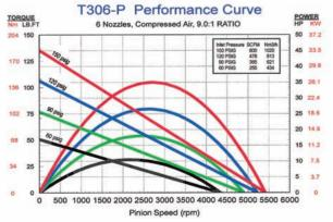
Lots of torque with low air flow sets T30 as the standard for cranking power in engines up to 20 liters.
