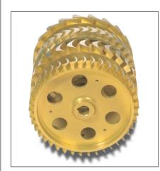
The large channels of TDI turbine blades create an open air path that allows contaminants to pass through rather than get lodged in the starter and cause breakdowns.
