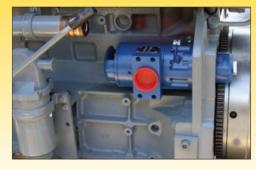
T20 installed on Deutz 1013 engine.
