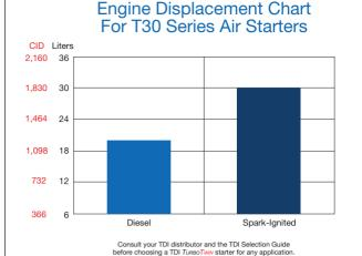
This selection chart shows basic starter capability by engine size. Note the chart shows four-stroke diesel engine size on the left and fourstroke, spark-ignited engine sizes on the right. Always consult TDI for applicationspecific capability.
