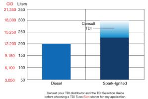
This selection chart shows basic starter capability by engine size. Note the chart shows four-stroke diesel engine size on the left and fourstroke, spark-ignited engine sizes on the right. Always consult TDI for applicationspecific capability.
