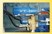
T100-F installed on Detroit Diesel 16V2000 engine.
