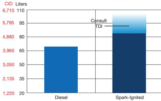
This selection chart shows basic starter capability by engine size. Note the chart shows four-stroke diesel engine size on the left and four-stroke, spark-ignited engine sizes on the right. Always consult TDI for application-specific capability.
