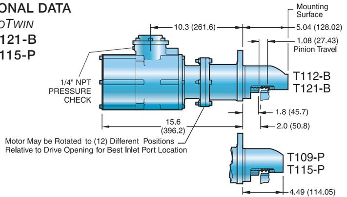
Motor May be Rotated to (12) Different Positions Relative to Drive Opening for Best Inlet Port Location
