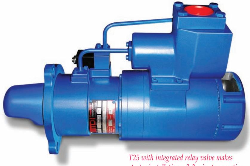
*T25 with integrated relay valve makes starter installation a 2-3 minute operation.*
