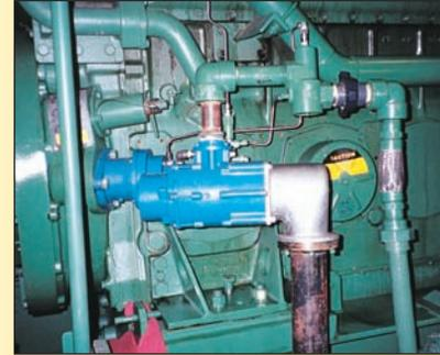
*The TurboTwin Model T100-V starter's offset and overhung pinion design provides a "bolt-on fit" to most large-displacement industrial engines. It installs in minutes when replacing other turbine-type starters. (Shown here on a Cooper Superior Series 2408G Spark-Ignited Gas Engine.)*
