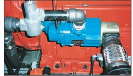
*Pressure check ports on both starter inlet and exhaust allow easy troubleshooting of compressed starting air/gas supply valves, filters, piping, and regulators. (Shown here TurboTwin Model T100-V and TurboValve.)*
